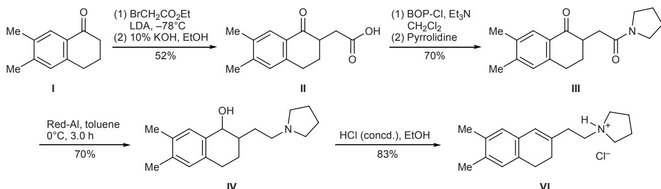
low cost and no need of isolating intermediate amine **V** (Scheme 1). The new synthetic procedure proposed by us consists of only four steps, and the overall yield is 21%, i.e., it is more efficient than the traditional methods. Moreover, the proposed procedure is suitable for enlarged syntheses.
